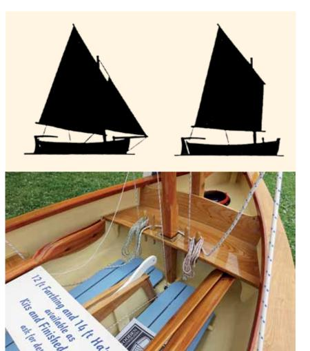
collar in the mast thwart acting as the adamant until you get hands-on, climb fulcrum, thus moving the CE forard and allowing the boat to be perfectly balanced when una-rigged. As you can see from the silhouettes, the mast is freestanding with running rigging only, which facilitates this manoeuvre. (A move from a sprit boom set-up to the balance lug would probably be effected onshore, not afloat.)
