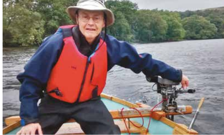
Seagull outboard and the reinforced wooden cross beam
