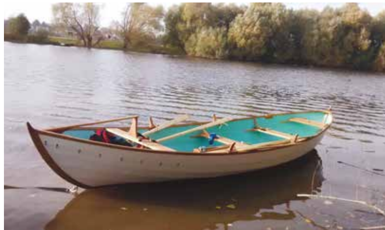
The wooden kabs can be seen in the rowing positions. The detachable support for the bow dodger is also visible
