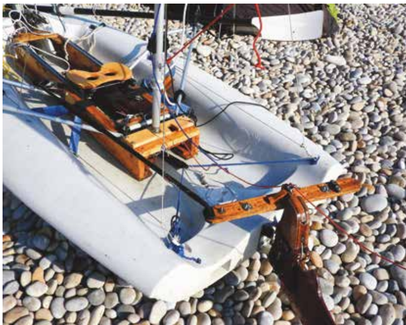
The PicoMicroYacht tiller system, designed to circumvent the mizzen mast
