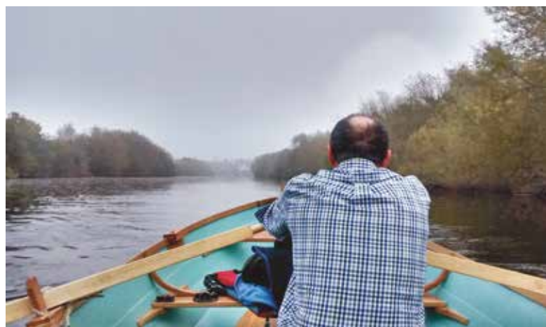
Note square section oars and thole pin with rope grommet
