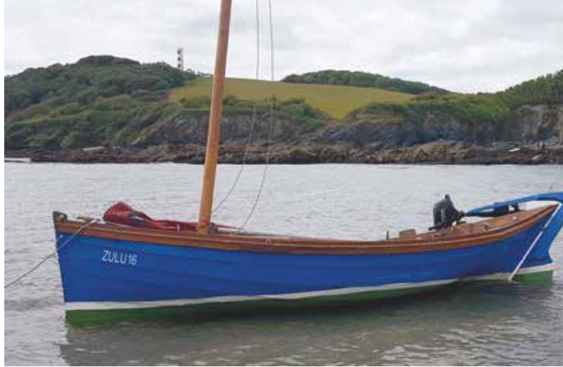
Matt and Rachel's 16-foot Zulu, with dipping lug rig
