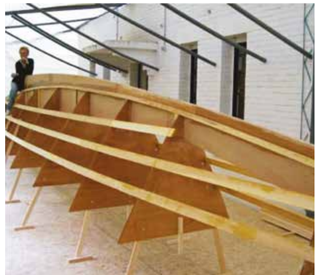
(Above) This is a sophisticated ocean-going Wharram cat in build, the Tiki 46 – but the basic construction is classic early Wharram. A plywood kelson is slotted into the bulkheads to give it longitudinal shape and strength. Being a big boat, it has an outside keel, too, unlike the Maui. The stringers and bulkheads provide crosswise strength. This hull is usually diagonally planked, as it is more rounded than the normal flat-sided Wharrams, which require plywood sheets to bend in one plane only
