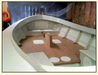
A view of the huge interior of Chip Matthews' PILGRIM, the buoyancy tanks under the seats and decks are sufficient to float the boat stable and upright even when fully swamped, an essential for an undecked boat that ventures into open waters. © Chip Matthews
