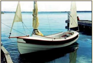
angles to rest the sore backs that so many of us suffer from, the seats are sealed to provide buoyancy, as is the raised deck area forward of midships that is large enough for the two of them to bed upon, and there is a huge locker under the foredeck where larger items can be stowed behind the hatch to keep them all dry.
