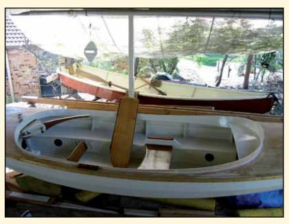
With the removable rowing seat and foot stretcher lifted out and stowed, WALKABOUT has a very nice comfortable space in which to lie down. Note that builder Wayne Jorgensen found that his WALKABOUT was faster under oars than the JW-designed SEAGULL behind, and that boat's no slug either.
