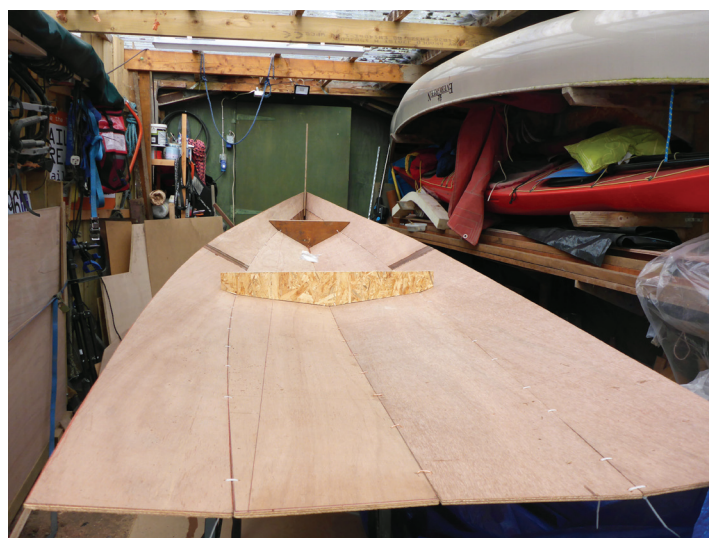
Photo 2: The first two strakes on each side are stitched together, with two simple formers to keep them open. The garboard strakes are the hardest to close at the bow as they have to twist through almost 90 degrees. I poured boiling water over the forward end of the garboard strakes to soften the plywood and pulled them together at the bow with a bolt and penny washers through both strakes.
