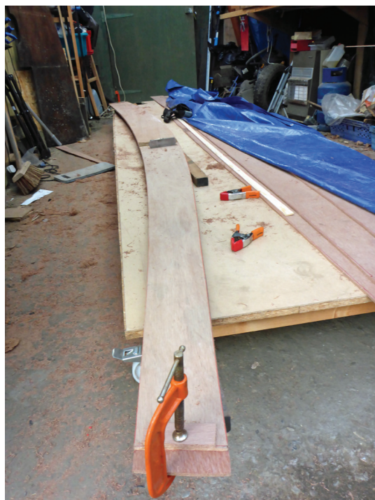
Photo 1: Planing the strakes to the line. The port and starboard strakes are clamped together to ensure they are perfect mirror images of each other
