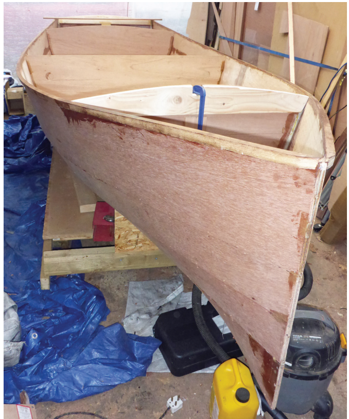
Photo 5: (above) The first outwale is on and the boat now feels much more rigid.
