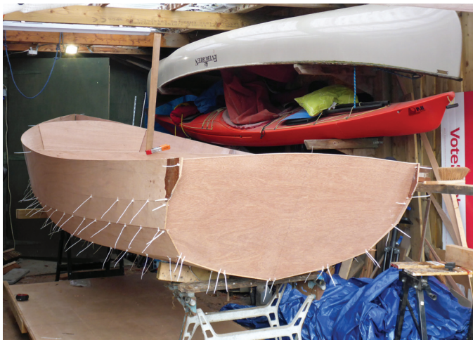
Photo 4: (below) And now the fourth (and widest) strake is on. It is split for about the first metre, to create tumblehome in the quarters. Suddenly, she has become a graceful boat!
