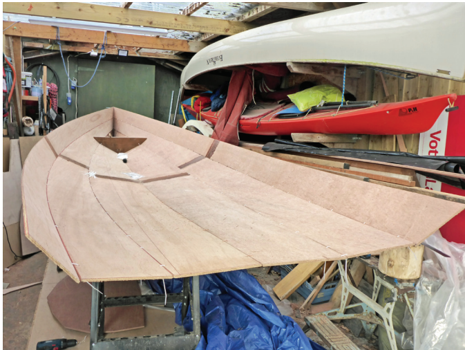
Photo 4: (below) And now the fourth (and widest) strake is on. It is split for about the first metre, to create tumblehome in the quarters. Suddenly, she has become a graceful boat!
