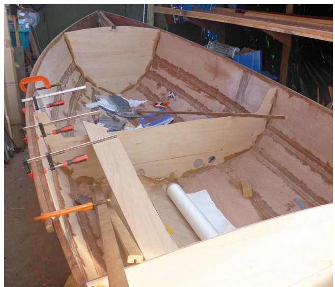
Photo 6: (below) The second outwale going on. The bow section has been epoxied, but the scarp still has to be cut in the aft end before the final section is pieced in. Once the inwales were in place the boat felt very robust.
