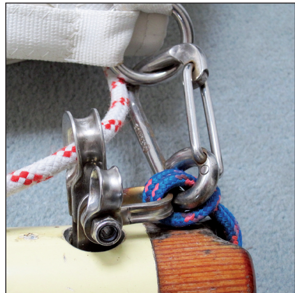
Boom tack fitting (sail not attached). Luff reef line passing through rounded shackle, not block. Strong Wichard snap hook shown attached to ring
