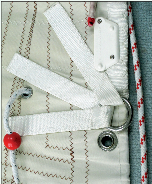
Luff reefing showing stainless ring attached with webbing and one reefing pendant bobble
