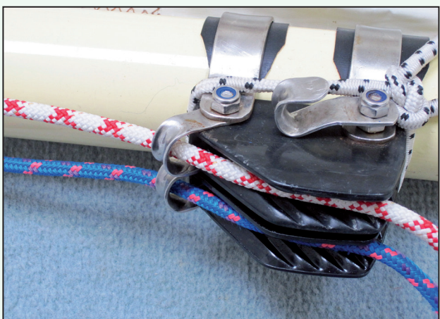
Strip shackles used to make fairleads for clam cleats, and hook
