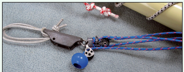
The business end of the boom mini-tackle, bungee tensioner unhooked for clarity
