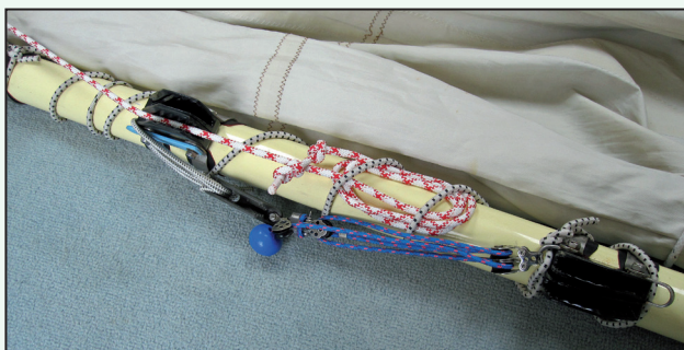
Reef line hauled and stowed in bungee spiral on boom
