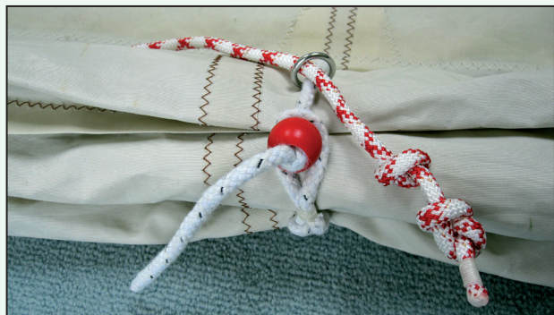
Leech line for Reef 2 now at boom level when Reef 1 is taken in
