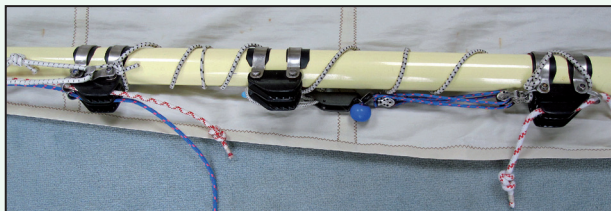
Battery of boom clam cleats showing (left) reef 2 leech line and clew outhaul control line in blue. (Right) luff reef line. All untensioned
