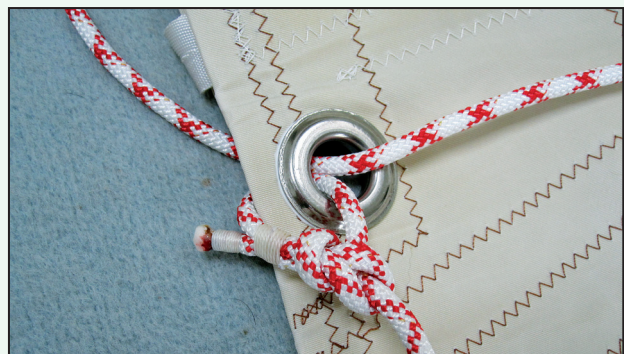
The upper (fixed) end of Reef 2 showing the line for reef 3 coming down sail leech and passing through cringle and passing forward across sail
