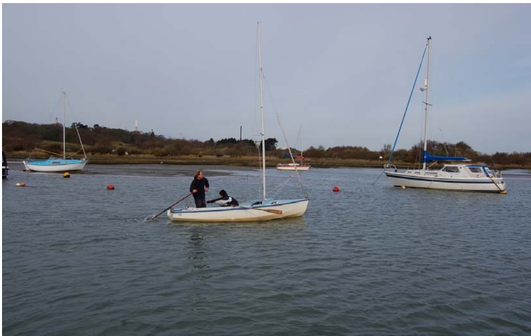
Sarah and I rowing our Wayfarer. The sculling oar is 8' 6" long with a blade 30" long and 4" wide. The blade meets the handle at an angle of 18 degrees.
